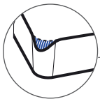
PLASTIC DEFORMATION (Thermal Wear)
